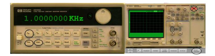
Once we have done this, the oscilloscope shows us the signal (see images below). In order to "read" the provided information we should adjust the time base (see black circle) and click again on *Perform experiment*. Now we can see that the vertical scale (see black circle) need to be adjusted and once again click on *Perform experiment*.
