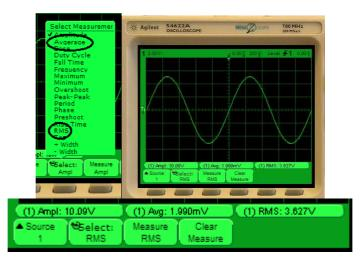
Now it makes sense to work with different signals in order to study which value is the most representative: the highest value (Vmax), the lowest value (Vmin), the distance between the highest and the lowest value (Vpp, Vpeak-to-peak), the mean value (Vcc, average), and the effective value (Vrms)? What is the effective value? Can you relate it to the statistical indicators?
