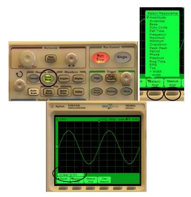
To measure the mean (average) and effective (RMS: root-mean-square) value we should repeat the previous steps. In this case the peak-to-peak value is 10.09 V, the mean value is 1.990 mV (i.e. nearly 0 V, the ideal or calculated value) and the effective value measured is 3.627 V, which is similar to 5/1.4142 = 3.5353 V.
