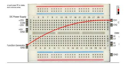
Now we should click on *Function generator* and select the type of signal, voltage and frequency. In our case, we are going to choose a sinusoidal signal of 10 Vpp and 1 KHz frequency, in both cases by turning the dial. When clicking on the oscilloscope, all we have to do is to click on button "1" and on *Perform experiment* (not on RUN or on SINGLE).
